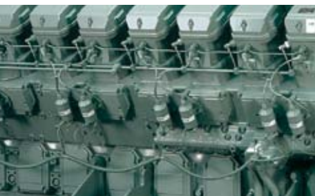
Spark ignited prechamber system
